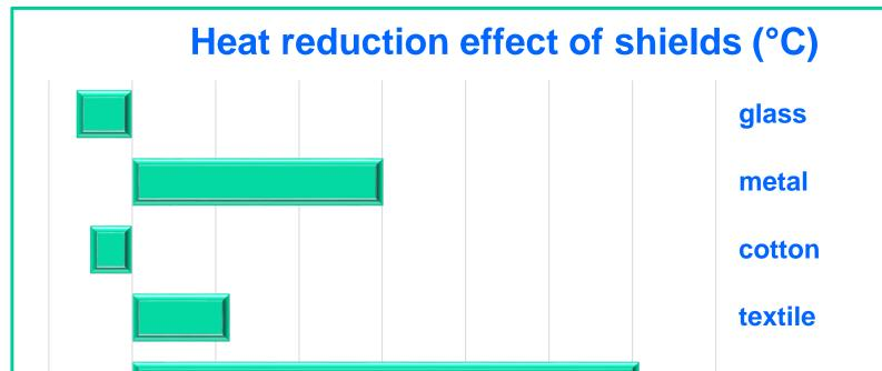
Our student-groups do independent measurements to test different materials for heat shield.
